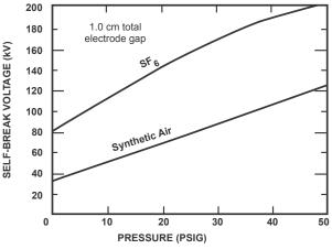
These curves depict the self-breakdown parameters of the T-670 switches in the two available gap options. The operating voltage should be approximately 75% of the self-breakdown levels. Triggering is accomplished by applying a voltage to the mid-plane electrode. The trigger pulse should be a minimum of 50% of the gap operating voltage - 100% is recommended.
