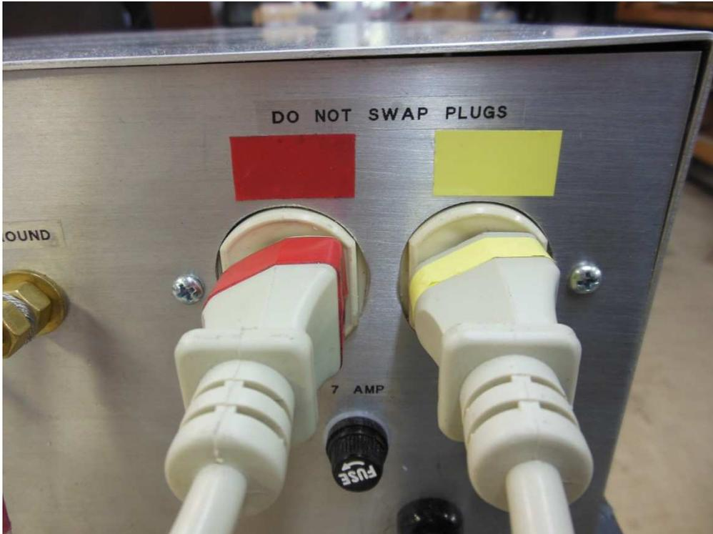
**FIGURE 5: REAR OF AMPLIFIER SHOWING OUTPUT CONNECTIONS**
