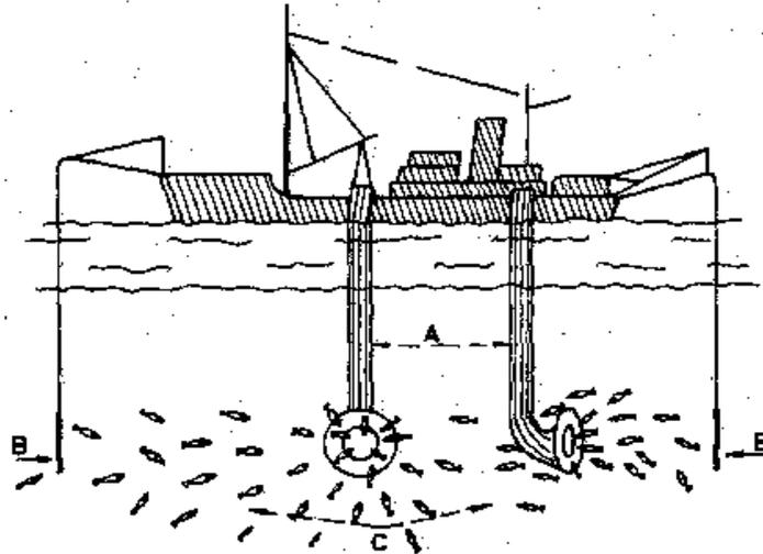
Fig. E14-6b. Diagram of electrical fishing (according to Skoskiewicz [3581]). A-Fish section pump; B-Electrode; C-Electrical field. By permission from P. F. Meyer-Waarden, "Electrical Fishing," Food and Agriculture Organization of the United Nations, 1937.
