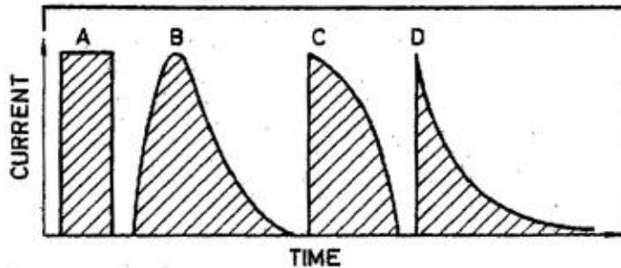
**FIG. E14-1. Various current impulses (according to Kreutzer [343]). A-rectangular pulse, B-unperiodic pulse, C-part of a sinus-curved pulse, D-capacitor discharge. By permission from P. F. Meyer-Waarden, "Electrical Fishing," Food and Agriculture Organization of the United Nations, 1957.**
