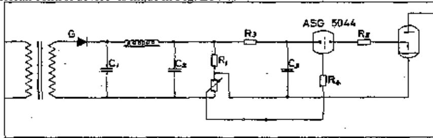
E14-7a. Diagram of a controlling device for Chinese crab or fish barriers. C<sub>1</sub>, C<sub>2</sub> and C<sub>3</sub>-capacitors; G-rectifier; R<sub>1</sub>, R<sub>2</sub>, R<sub>3</sub>, R<sub>4</sub> and R<sub>6</sub> rheostats; ASG-ignifron. By permission from P. F. Warden, "Electrical Fishing," Food and Agriculture Organization of the United Nations, 1957.
