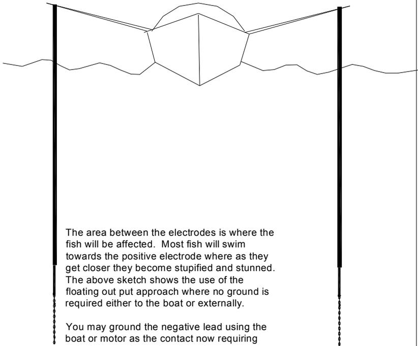
The area between the electrodes is where the fish will be affected. Most fish will swim towards the positive electrode where as they get closer they become stupified and stunned. The above sketch shows the use of the floating out put approach where no ground is required either to the boat or externally.
