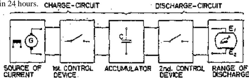
Fig. E14-6a. Basic principle of producing impulse current (according to Haier 1334). By permission from P. F. Meyer-Waarden, "Electrical Fishing," Food and Agriculture Organization of the United Nations, 1957.
