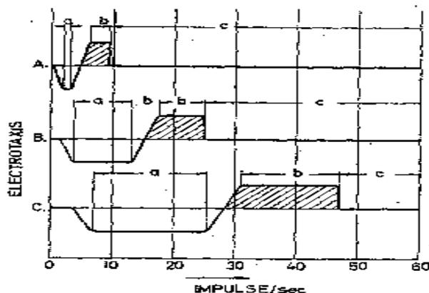
Fig. E144. Influence of impulses per second on various fish (according to Kreutzer [343]). A-tuna, B-cod, C-herring. (a) Possibility of escaping, (b) Swimming towards the anode, (c) Electro narcosis. By permission from P. F. Meyer-Waarden, "Electrical Fishing," Food and Agriculture Organization of the United Nations, 1957.
