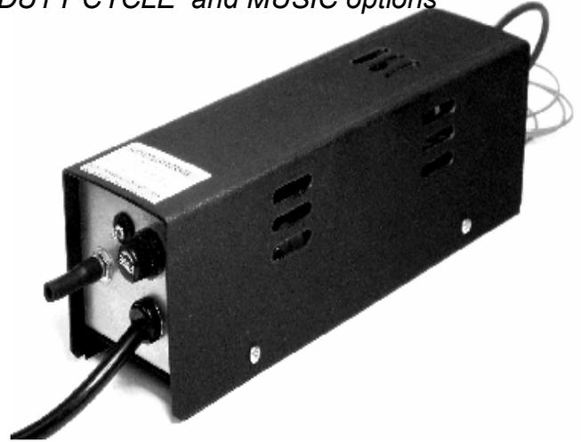
On/off power control has an insulating shaft extension to prevent annoying burns
