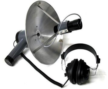
1. Slide off plastic cap located on handle and install 8 aa batteries in the holder. Make sure batteries are making contact as some holders are very tight. You may use a single 9 volt but headphone volume will be reduced. Replace cap.
